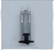
W Series "SERIES TRIP", "PUSH TO RESET" Single Pole circuit breakers represent our largest selling product family. Bases on a proven "SNAP ACTING" bimetallic thermal seneing elemant system. W Series circuit breakers sease Overload conditions and interupt the flow of Current. The resettable actuator mechanism then remains disengaged until manually reset.
